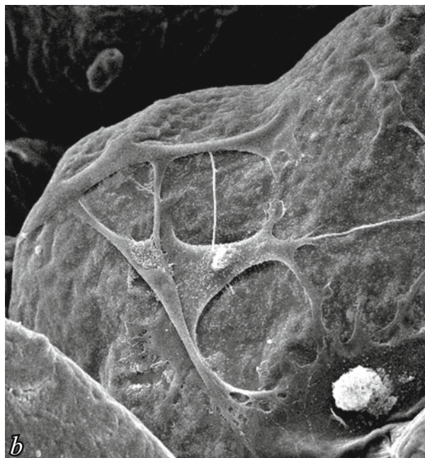
Fig. 3. MSC adhesion on the surface of polylactide carriers after 3-day culturing (SEM, \times 600 ). (a) individual cells; (b) clusters of cells.
